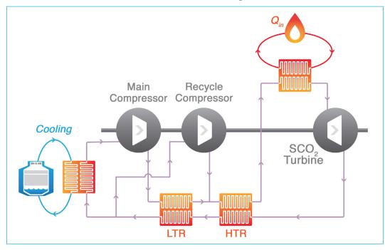
Closed Loop SCO<sub>2</sub> Recompression Brayton Cycle Flow Diagram
